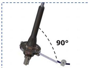
The furling line should be installed as shown on the drawing.
